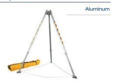
Extruded aluminum 2-stage adjustable legs provide 5' to 8' working height, includes two head-mounted pulleys and two anchoring auxiliary eyebolts, leg-securing safety chain and steel feet with non-slip pads. Offers 55" to 91" internal working height and includes 70" storage bag.
