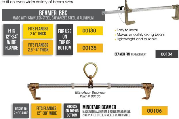
Featuring the same high performance and durability of Guardian's other Beamer products, the *Minotaur Beamer* is specially designed for attachment to wider beam flanges.
